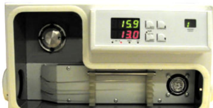
**Figure 1-2. Front view of the column chamber showing the column inlet and outlet fittings.**
